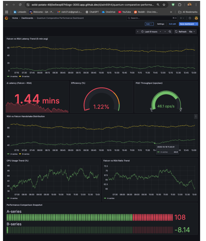
Fig. 8. Comprehensive Performance Dashboard—aggregated latency, throughput, and CPU metrics contrasting classical and PQC pipelines.
